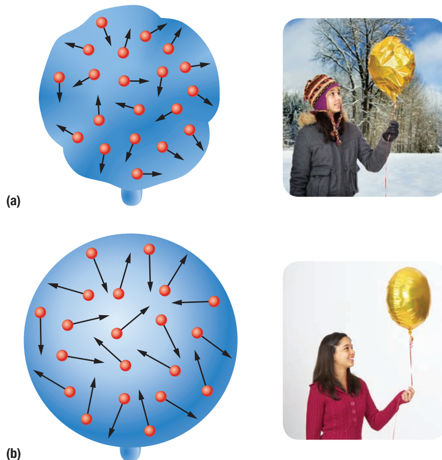
Figure 3 The helium gas in a mylar balloon expands a great deal when the balloon is taken from the cold outdoors into a warm room.
